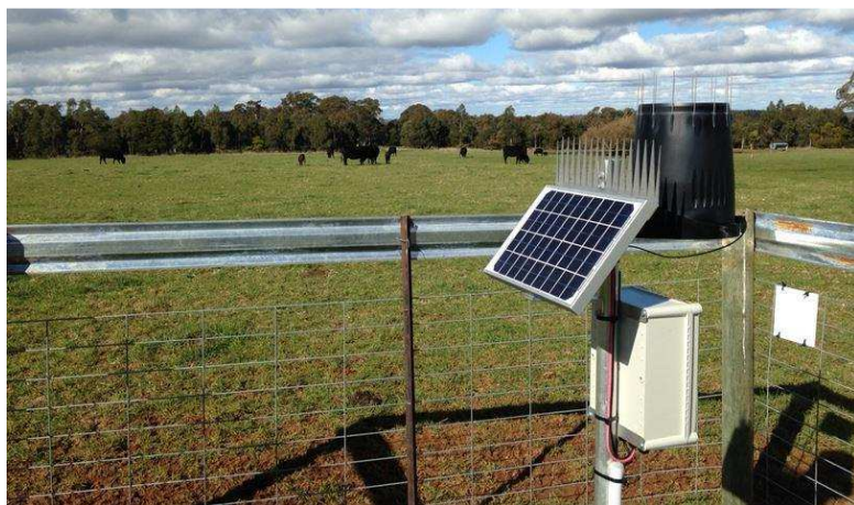
Image: Soil moisture logger recording real-time information on an improved pasture at Bannister (M. Lieschke, South East Local Land Services).
