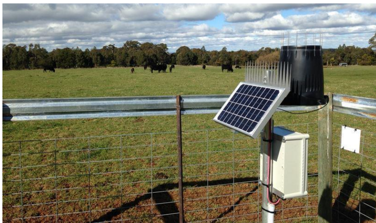
Image: Soil moisture logger recording real-time information on an improved pasture at Bannister (M. Lieschke, South East Local Land Services).
